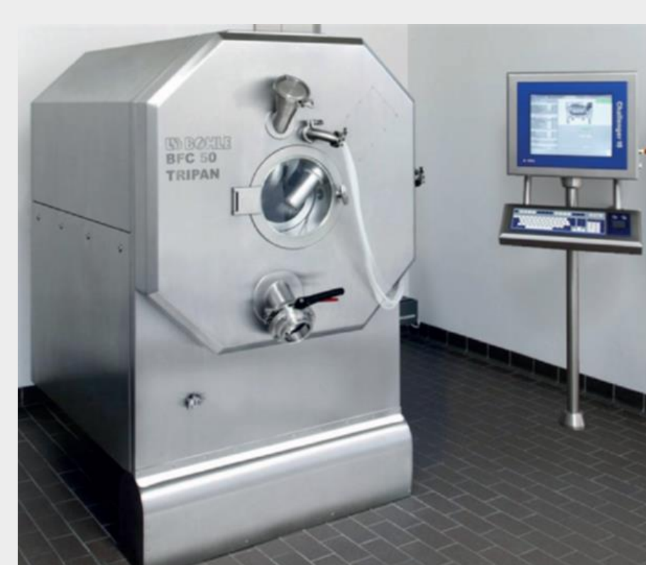
Figure 1: Coating trials were conducted in a BFC 50 tripan full perforated coating pan (L.B. Bohle, ennigerloh, Germany) equipped with six spray nozzles (type 970, schlick, Germany) with a batch size was 20 kg.
